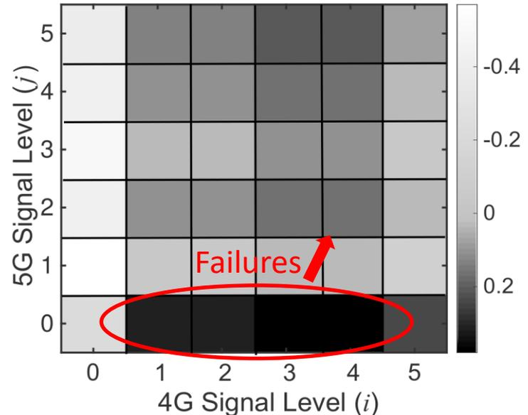
Increase of normalized prevalence of cellular failures.
