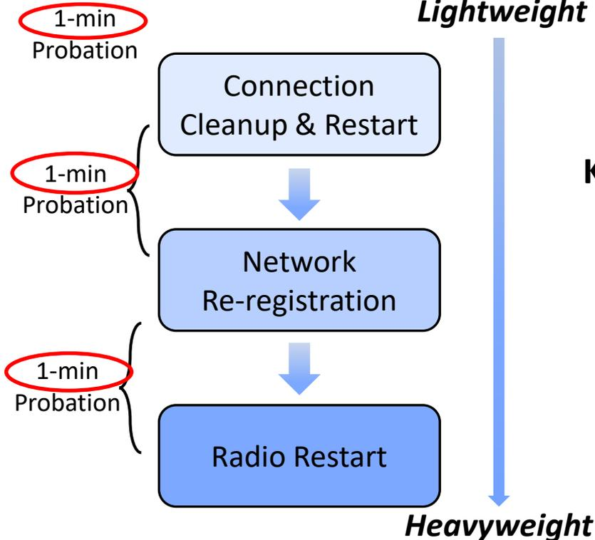
Android's *three-stage progressive* mechanism for Data\_Stall Recovery
